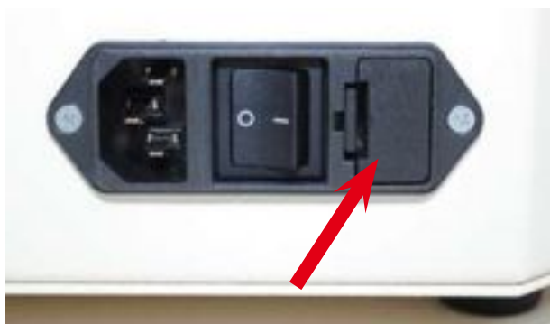
Main switch with fuse box on the rear panel.
