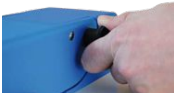
Pulling out the locking mechanism
