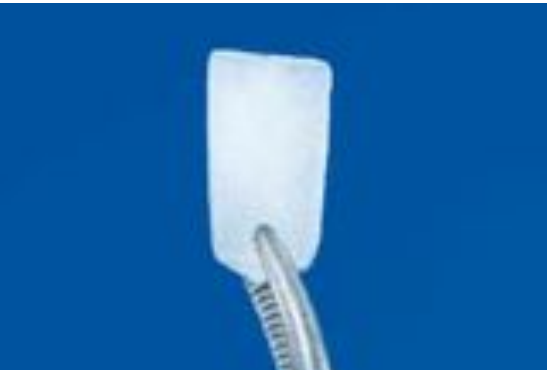
Fig. 1a: Bake specimen, temperature too low.
