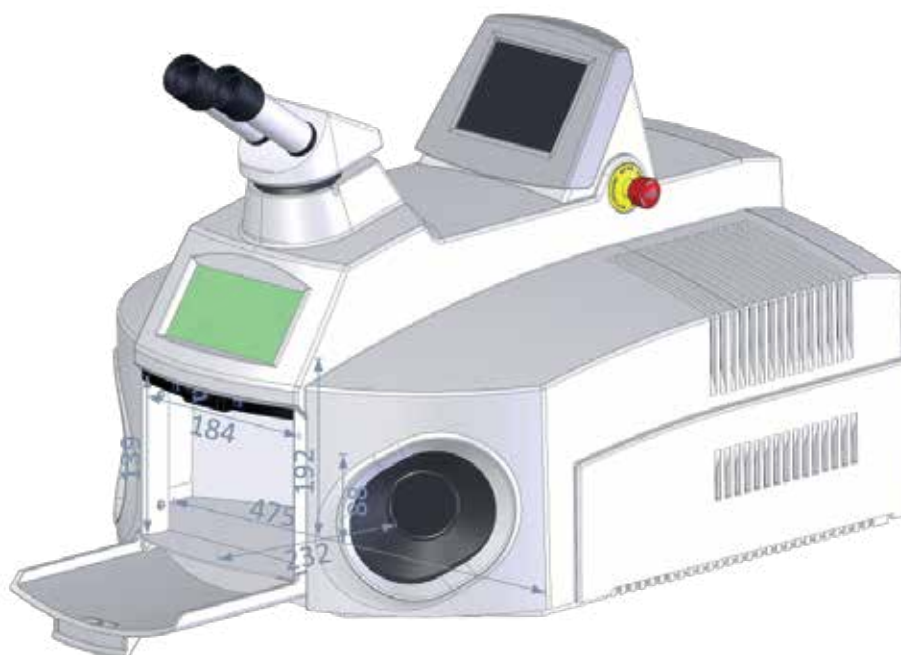
Figure 6: Working chamber dimensions
