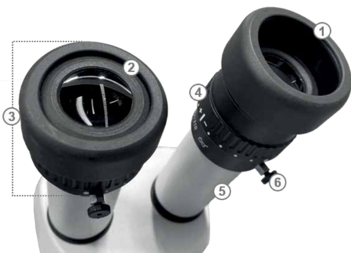
Figure 18: Ocular and eyecups of the Leica microscope attachment
