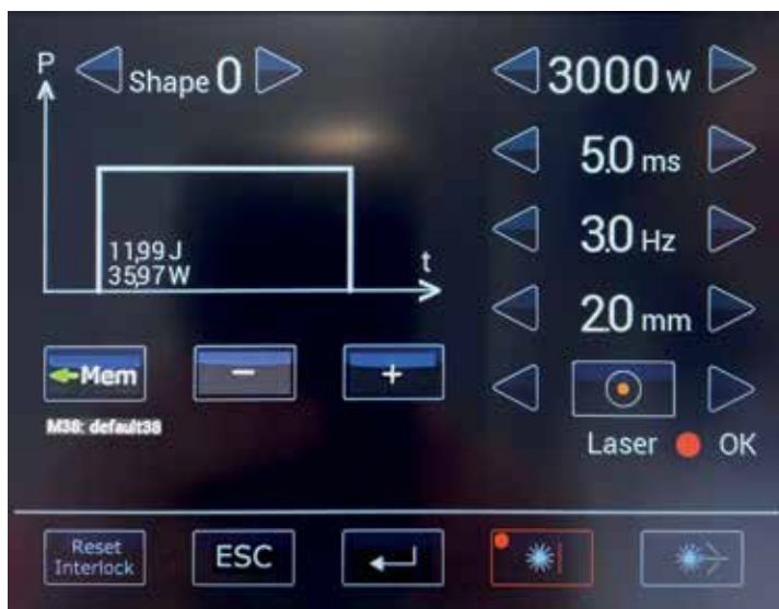
Figure 15: Touchscreen main window – in load parameter set mode
