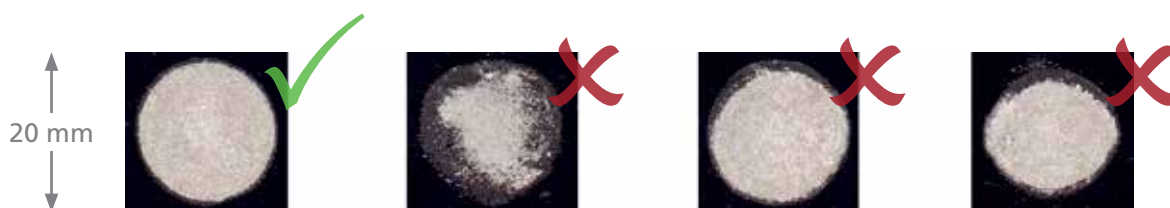
Figure 26: Focal spot impression on photographic paper
